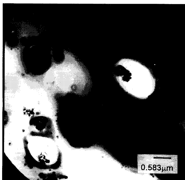
Figure 2 Transmission electron micrographs of polypyrrole/EPDM semi-IPN prepared using 33% CuCl 2 (<105 μm) and 0.8% dicumyl peroxide (24 h polymerization time). Magnification = 12000
